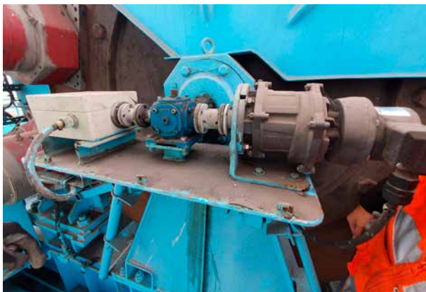
Old solution with distribution gear.
