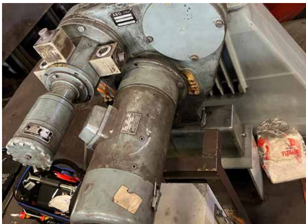
Original installation with a distribution gear, tachometer and overspeed switch.
