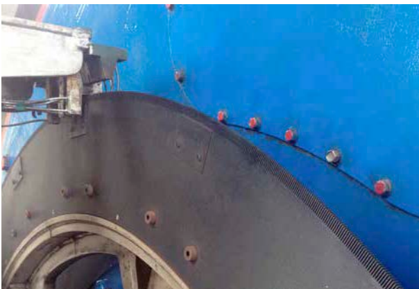
Before: The resolution of the existing inductive tooth wheel scanning solution is no longer sufficient for high-precision speed control.
