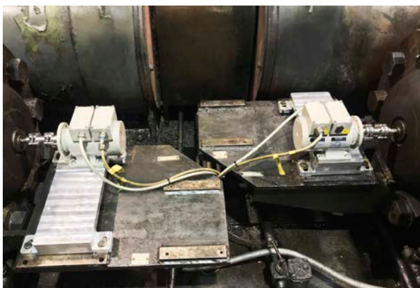
After: Directly attached electronic position switch ERC 40 with an additional current output for up-to-date position monitoring.
