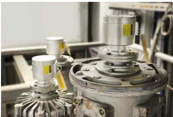
After: Incremental encoder facilitates digital speed control.
