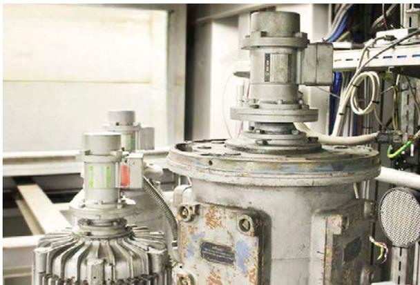
Before: Speed monitoring with analog tachometer generators.
