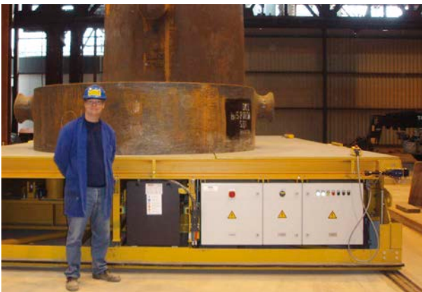
Heavy-load transporters are used to transport the casting ladles from the warehouse to the casting house.
