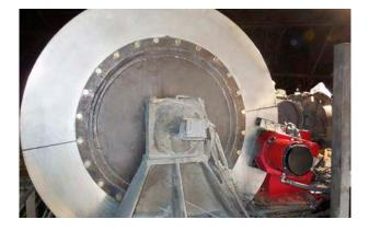
Before: Hoist drum with mechanical rotary cam limit switch, but without overspeed detection. Bottom right, the new holding brake.
