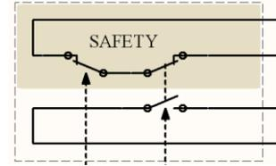
A separate diagnostics switch (Diag) closes when no errors are diagnosed. This is also indicated on the front of the module by a green LED. If an error is established the switch opens and a red LED lights up.
