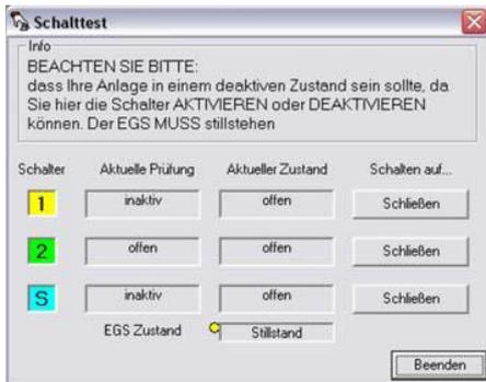
If the device is at a standstill all switches can be activated separately and thus can be checked for function.
