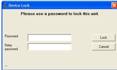
The EGS®40 can be safeguarded against unauthorized write access via a device password. The device password is stored in the read-only memory of the respective connected device.
