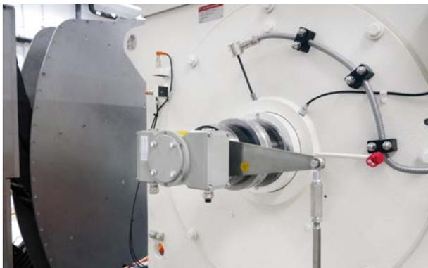
*Overspeed switch EGSHJ 41 from Hübner Giessen including attachment incorporating fault exclusion for reliable speed monitoring at the test stand motor.*
