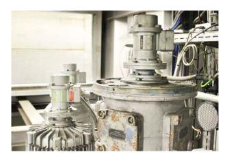
Before: Speed monitoring with analog tacho generators.
