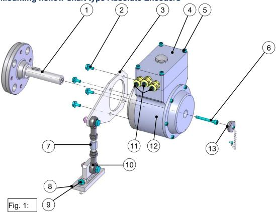
1. Mount adapter shaft (1) and align using dial gauge.
