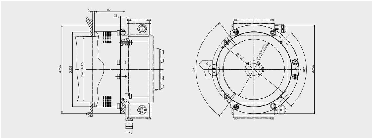
**System solution** Cover on FGH 6 / adapter shaft
