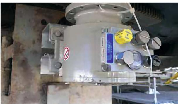
挖掘机/回转齿轮: 绝对值编码器 AMPN 41 (PROFIsafe via PROFINET, SIL 3/PL d)
