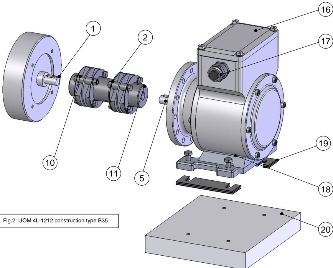
Fig.2: UOM 4L-1212 construction type B35
