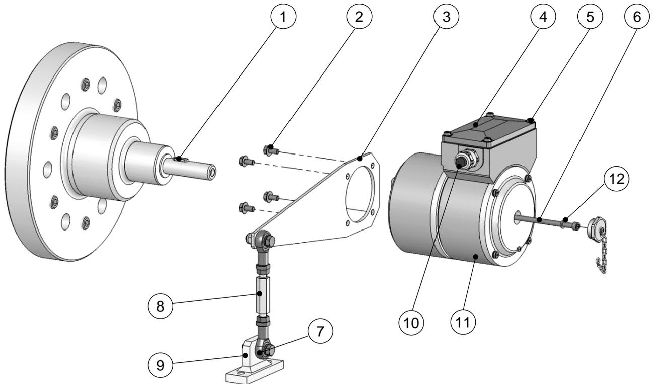
1. Mount adapter shaft (1) and align using dial gauge.
