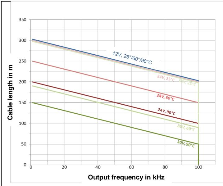
Fig. 5: Maximum permissible cable length for HTL interface
