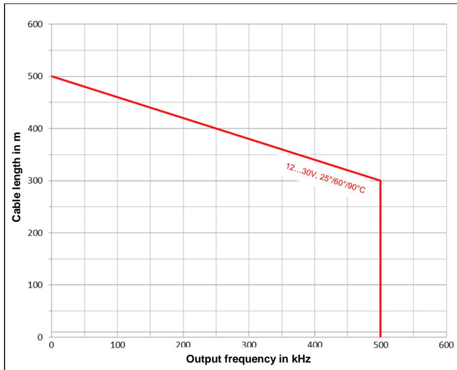
Fig. 3: Maximum permissible cable length for SIN/COS interface
