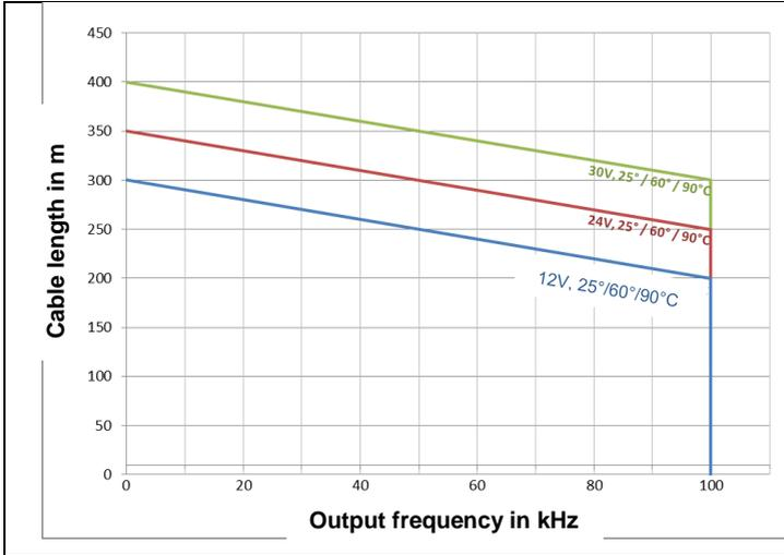
Fig. 4: Maximum permissible cable length for TTL interface
