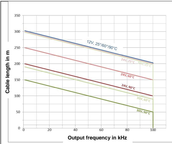
Fig. 3: Maximum permissible cable length for HTL interface
