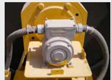
U-ONE® Multiturn Basisgerät Seiltrommel U-ONE® Multiturn basic unit installed at rope drum
