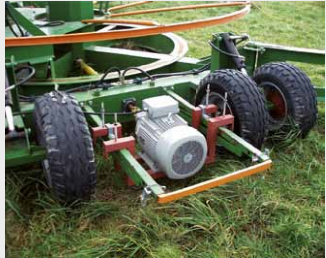
Mobile wind energy converter Mowec with generator DSG P 160.20-10
